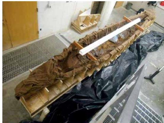
**After casting, the concrete canoe had to be checked twice daily for 28 days. The team devised a system of a plastic, burlap, humidifiers, and periodic misting with a hose to keep the concrete in its ideal conditions.**
